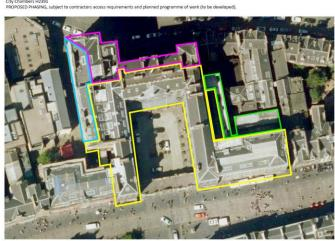
Yellow - phase 1, general areas, roof and higher elevation levels. Blue - phase 2 - all. Magenta - phase 3 - all. Green - phase 4 - lower elevations and lower roof levels
